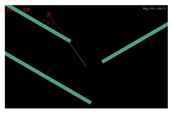
A line will be drawn to represent the ray. Point one will be the centre of the screen and point two will be mouse position. So you can move the ray around.
