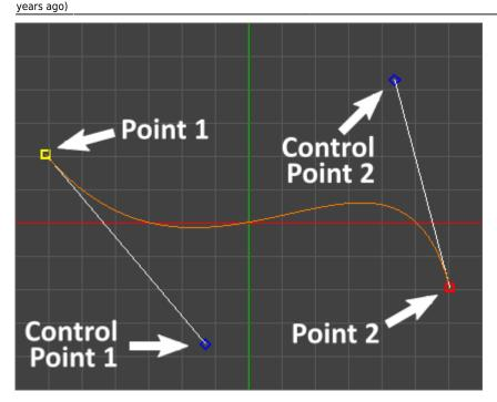
This tutorial centers around the use of the orxVector\_Bezier function. This function takes four vectors, 2 for the points, and 2 for the control points. The signature of the function looks like this:
