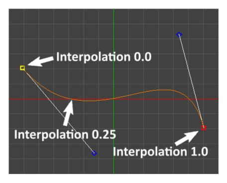
In the image above, by setting 0.25 as the interpolation position, you will locate a vector position a quarter of the way along the curve segment.
