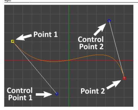
This tutorial centers around the use of the orxVector\_Bezier function. This function takes four vectors, 2 for the points, and 2 for the control points. The signature of the function looks like this:
